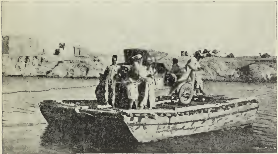
Ferrying the cars across the Euphrates. The cars were ferried across on flat-boats guided by wire cables, for at this point the current is very swift.
